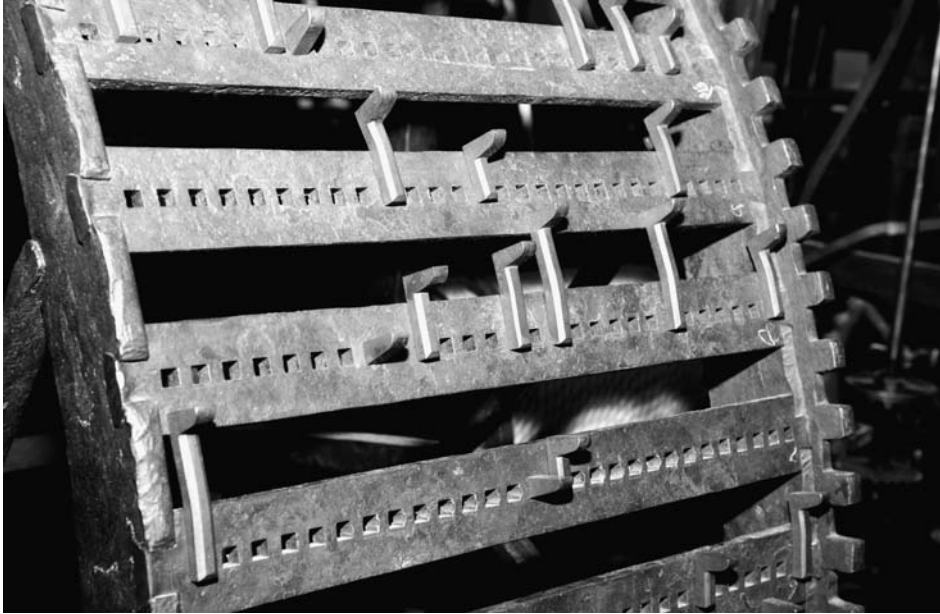
Playing drum, constructed by Hans Neurenberg for the New Reformed Church in Hattem, the Netherlands (1635). This is one of the last examples of a drum with slats in wrought iron.
