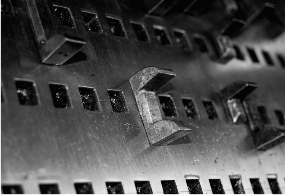
Pins on the drum of the city carillon of Antwerp
